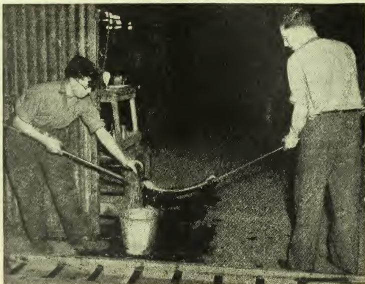
A worker (left) fixes a "post" to the finished ball prior to drawing
